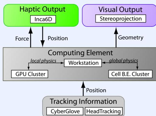
Figure 2: different components of the VR-System
