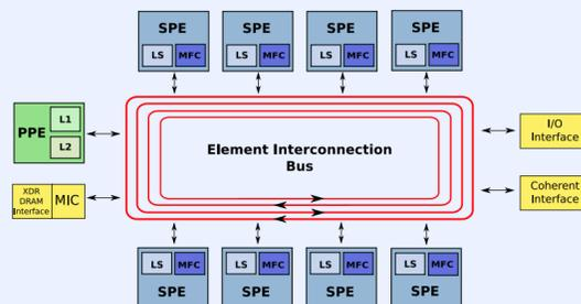
Figure 3: Cell B.E. Processor Architecture
