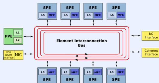
Figure 3: Cell B.E. Processor Architecture
