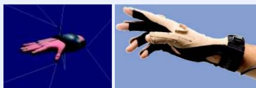
Figure 4: (left) wristband endeffector (right) CyberGlove
